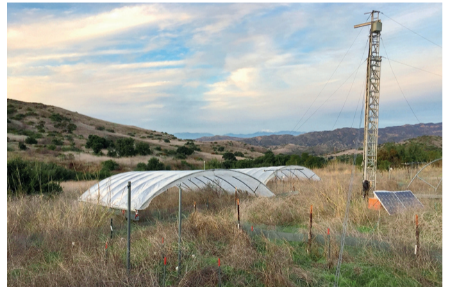
STAYING ALIVE: Studies of climate change impacts on soil microbes were conducted recently at the Loma Ridge Global Change Experiment in Irvine, California, where plastic covers reduced rainfall in order to reach experimental drought plots by nearly 50%. Interestingly, the microbial communities managed to survive the climate shock
